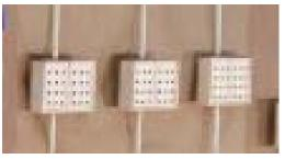
The target boxes supplied with the Creedmoor Air Rifle Target Systems that are used on many JROTC ranges use a steel plate (1) to stop fired pellets and drop them to the bottom of the box. They also employ a backing card in the middle of the box (2) to prevent lead fragments or residues from exiting the target box.
